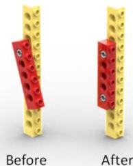
Fixing of Movable Structure
